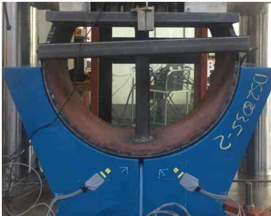
Figure 34: Crush testing of a composite pipe support
