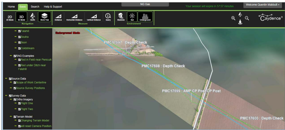
Figure 5: LiDAR Web Portal Presentation (showing the pipeline superimposed on the topographical LiDAR corridor, pipe sections are colour coded according to depth to aid analysis)
